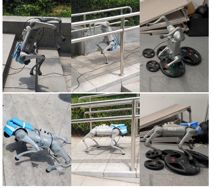
Fig. 3: Our policy deployed on a quadruped robot performs bipedal locomotion and quadrupedal locomotion over rough terrains. Upper row shows bipedal locomotion on stairs, slopes and discrete obstacles respectively. Lower row shows quadrupedal locomotion on stairs, slopes and discrete obstacles respectively.
